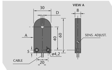
**MODELS WITH CABLE****SIA 05 - NE****SIA 12 - NE****SIA 15 - NE**
