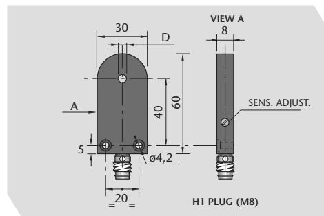
**MODELS WITH CONNECTOR****SIA 05 - NE H1****SIA 12 - NE H1****SIA 15 - NE H1**
